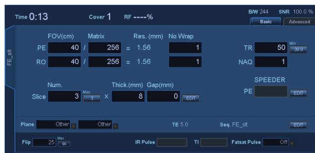
FE\_slit, Special Plan (Axial:1, Sagittal:1, coronal:1), TR50, NS3, ST 8 mm, Flip25, FOV 40 cm, MTX 256 × 256, NoWrap RO1.0/PE1.0
