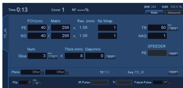
FE\_slit, Special Plan (Axial:1, Sagittal:1, coronal:1), TR50, NS3, ST8 mm, Flip25, FOV40 cm, MTX 256 × 256, NoWrap RO1.0/PE1.0
