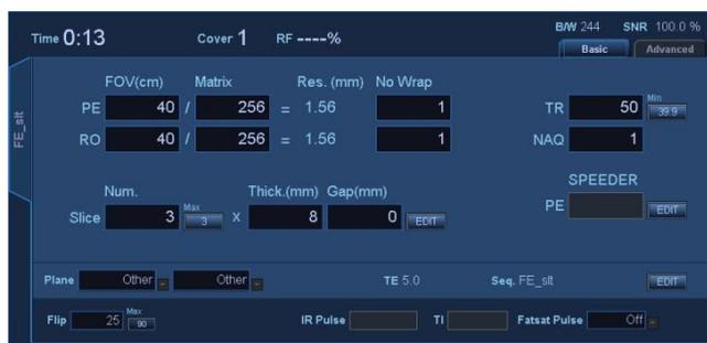
FE\_slit, Plano especial (Axial:1, Sagital:1, coronal:1), TR50, NS3, ST 8 mm, Flip25, FOV 40 cm, MTX 256 × 256, NoWrap RO1.0/PE1.0
