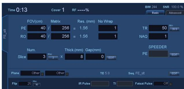
FE\_slt, Plano especial (Axial:1, Sagital:1, coronal:1), TR50, NS3, ST 8 mm, Flip25, FOV 40 cm, MTX 256 × 256, NoWrap RO1.0/PE1.0
