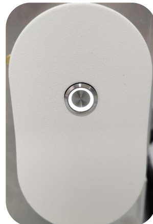
Power is on (light is on).
